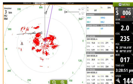
AIS vessels on a radar panel
